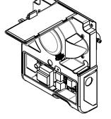
FIGURE 7. DH-100 ACCESS HATCH COVER TEMPORARY STORAGE
